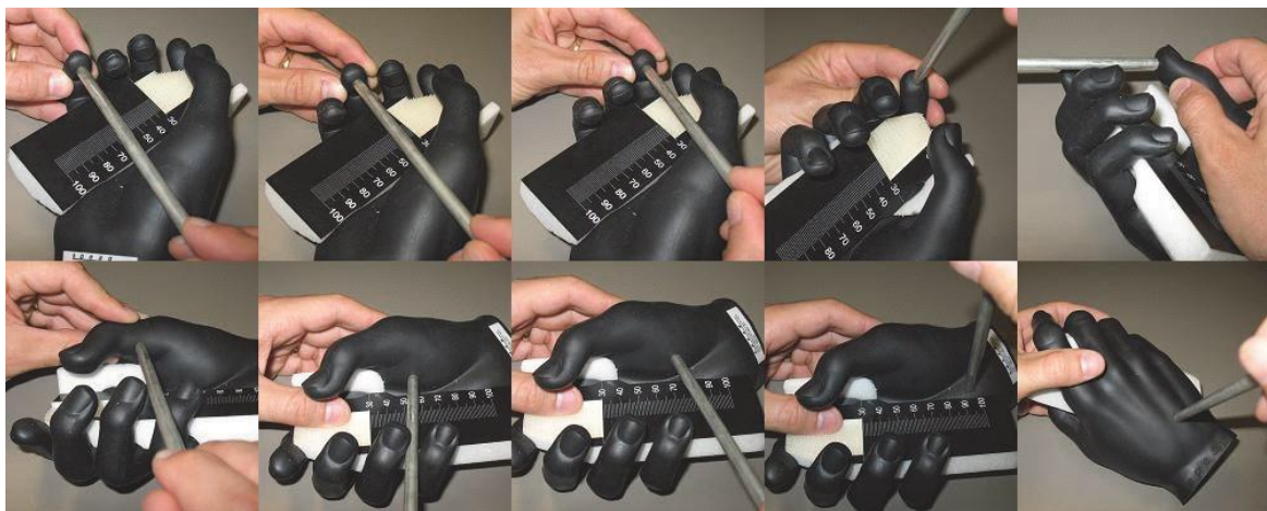
Figure 2.13.2.3-3 Ten Locations of Dielectric Measurements at the Narrow Data Hand Surface
