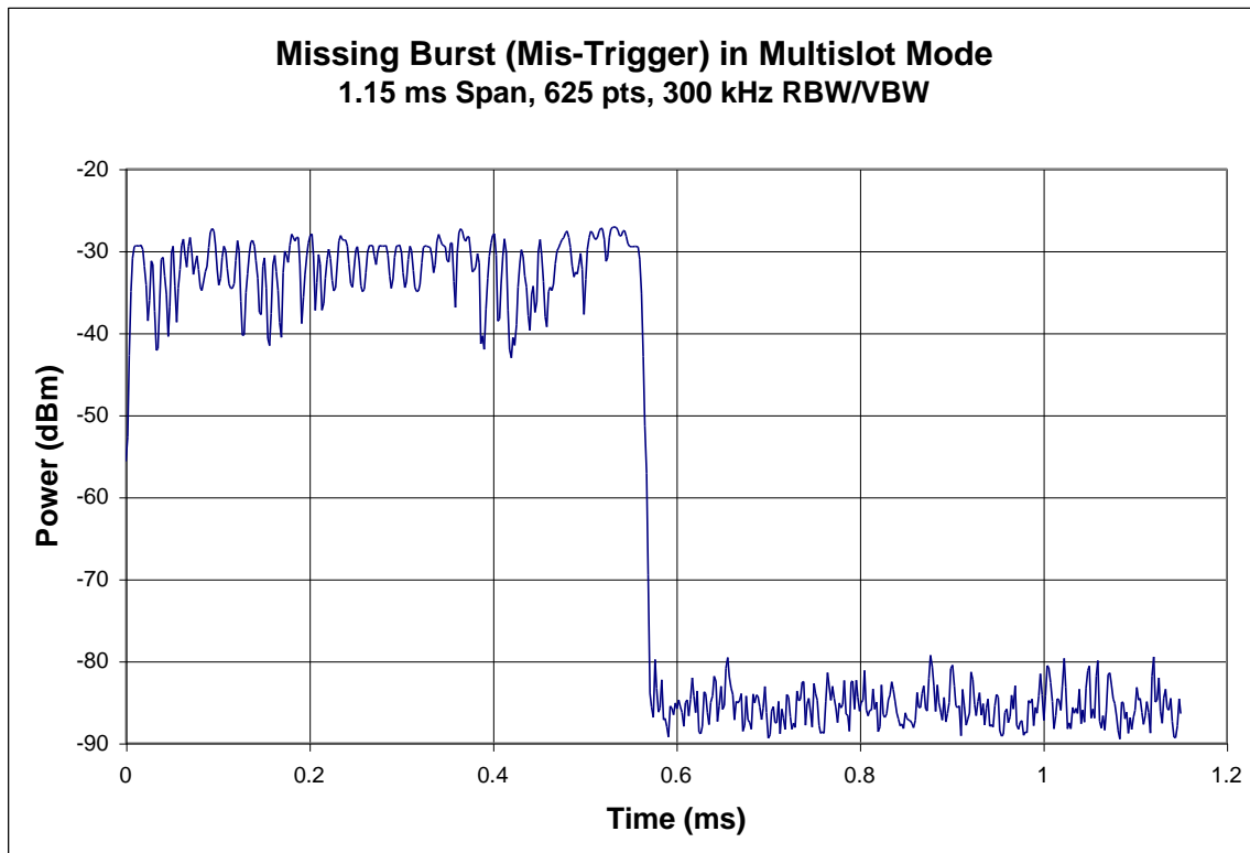
Figure 9.8-7 Bad 8-PSK Multislot Trace Resulting from Mis-Triggering
