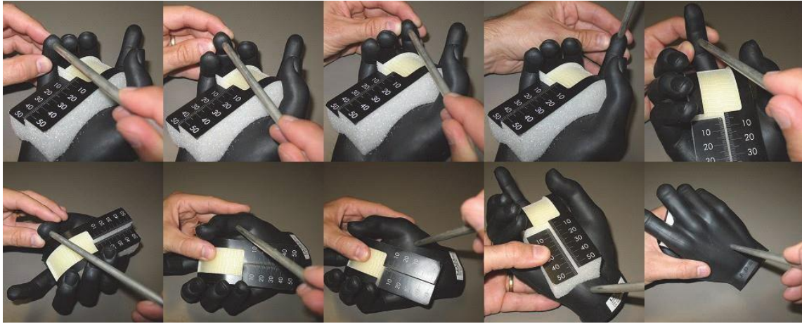
Figure 2.13.2.2-2 Ten Locations of Dielectric Measurements at the Fold Hand Surface
