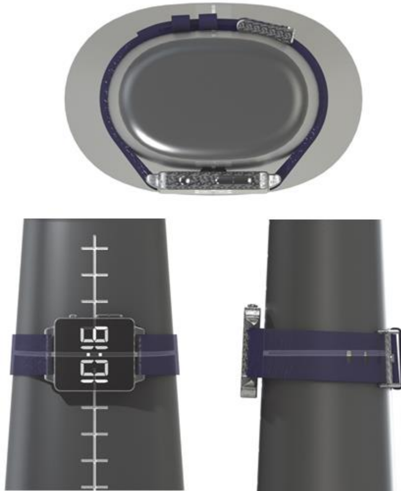
Figure 2.3.2-7 Examples of Correctly Mounting the Device on the Forearm Phantom by Keeping the Main Module Parallel to the Surface of the Forearm Phantom
