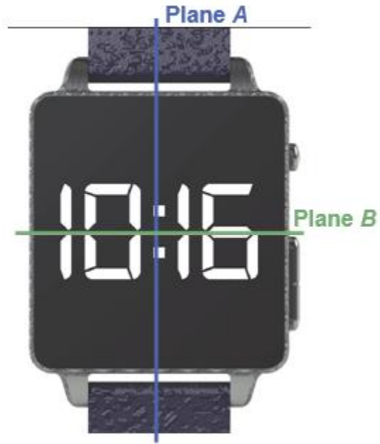
Figure 2.3.2-3 Definition of Plane A and Plane B on a Wrist-worn Device
