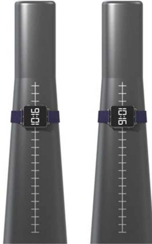
Figure 2.3.2-9 Two Orientations of DUT On Forearm Phantom Representing the Left and Right Wrist
