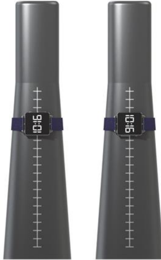
Figure 2.3.2-9 Two Orientations of DUT On Forearm Phantom Representing the Left and Right Wrist
