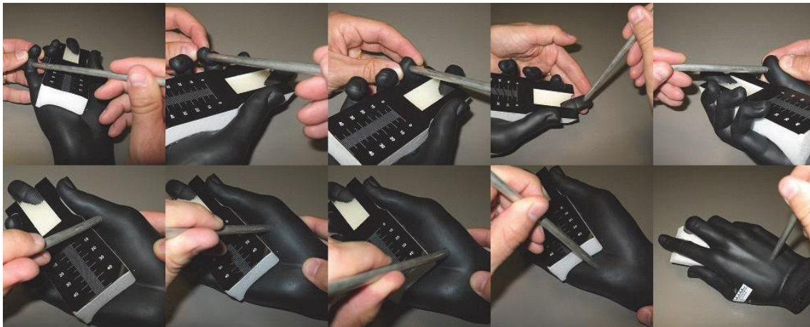
Figure 2.13.2.2-1 Ten Locations of Dielectric Measurements at the Brick Hand Surface
