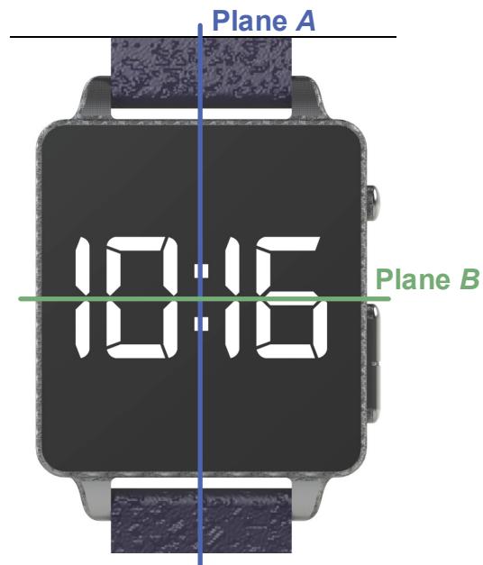
FIGURE Q-5 DEFINITION OF PLANE A AND PLANE B ON A WRIST-WORN DEVICE
