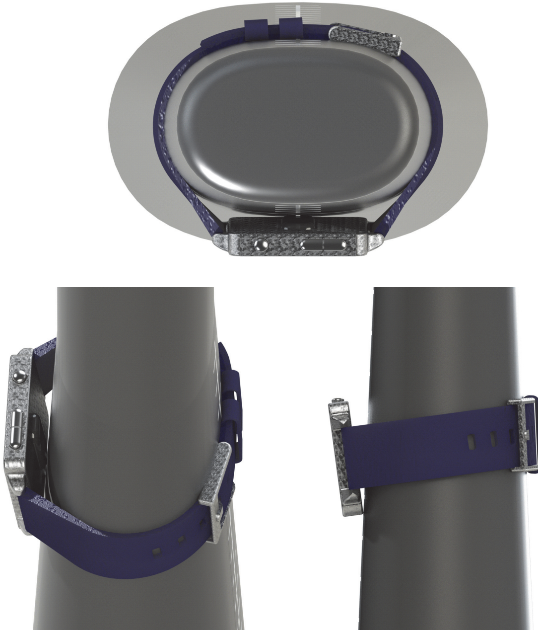
FIGURE Q-10 EXAMPLE OF INCORRECTLY MOUNTING THE DEVICE ON THE FOREARM PHANTOM BY NOT KEEPING THE MAIN MODULE PARALLEL TO THE SURFACE OF THE FOREARM PHANTOM
