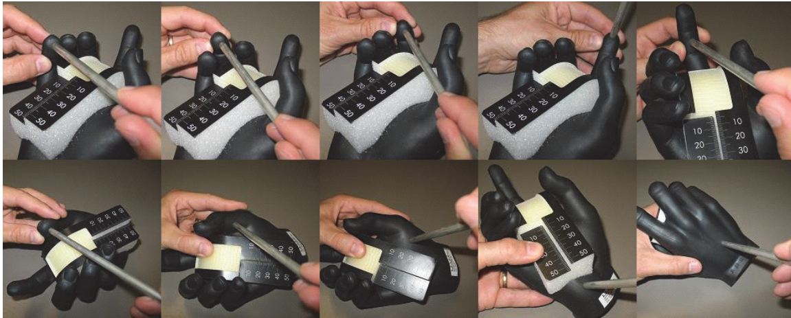
FIGURE G-2 TEN LOCATIONS OF DIELECTRIC MEASUREMENTS AT THE FOLD HAND SURFACE
