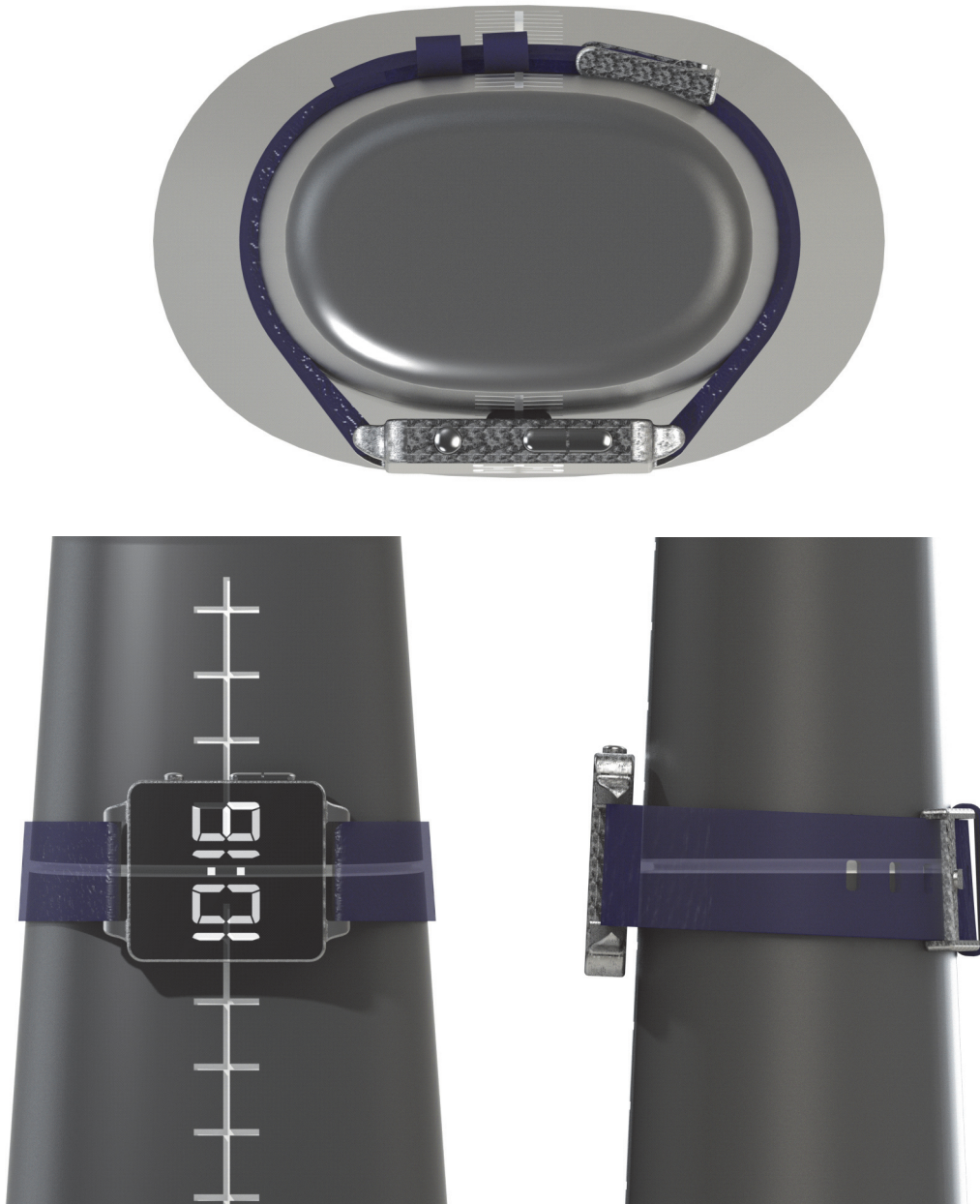
FIGURE Q-9 EXAMPLES OF CORRECTLY MOUNTING THE DEVICE ON THE FOREARM PHANTOM BY KEEPING THE MAIN MODULE PARALLEL TO THE SURFACE OF THE FOREARM PHANTOM
