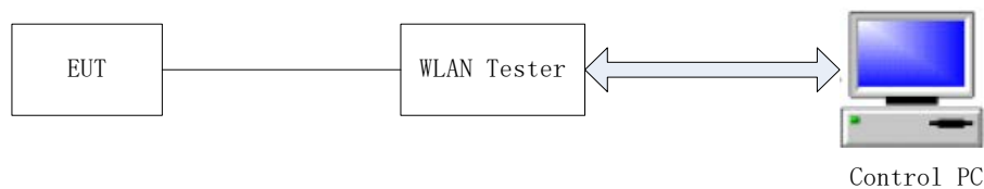
FIGURE 3.1-1 BLOCK DIAGRAM FOR WI-FI CONDUCTED MEASUREMENT
