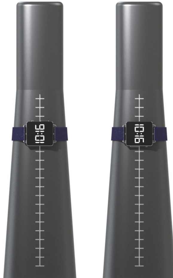
FIGURE Q-11 TWO ORIENTATIONS OF EUT ON FOREARM PHANTOM REPRESENTING THE LEFT AND RIGHT WRIST
