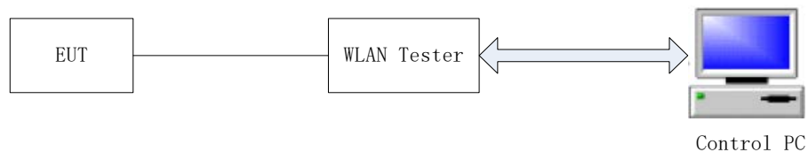
FIGURE 3.1-1 BLOCK DIAGRAM FOR WI-FI CONDUCTED MEASUREMENT
