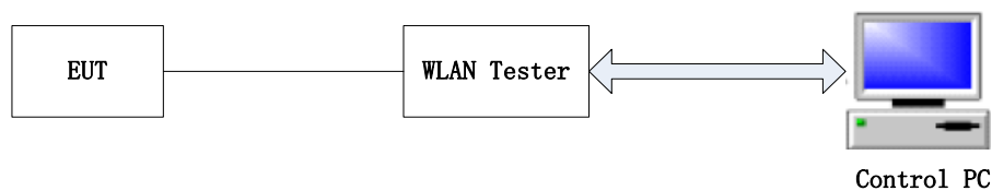
FIGURE 3.1-1 BLOCK DIAGRAM FOR WI-FI CONDUCTED MEASUREMENT
