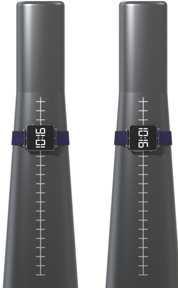
FIGURE Q-11 TWO ORIENTATIONS OF EUT ON FOREARM PHANTOM REPRESENTING THE LEFT AND RIGHT WRIST
