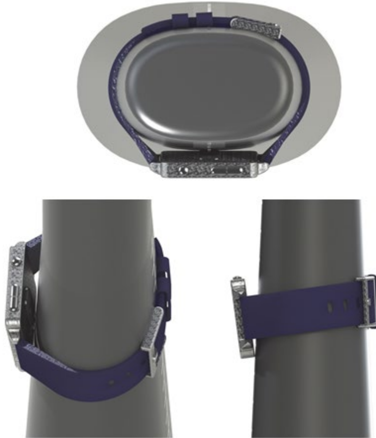
Figure 2.3.2-8 Example of Incorrectly Mounting the Device on the Forearm Phantom by not Keeping the Main Module Parallel to the Surface of the Forearm Phantom
