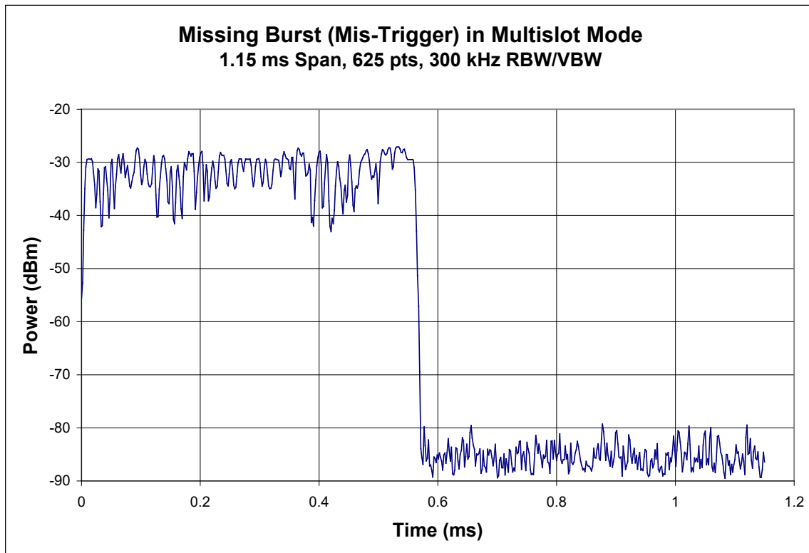
Figure 9.8-7 Bad 8-PSK Multislot Trace Resulting from Mis-Triggering
