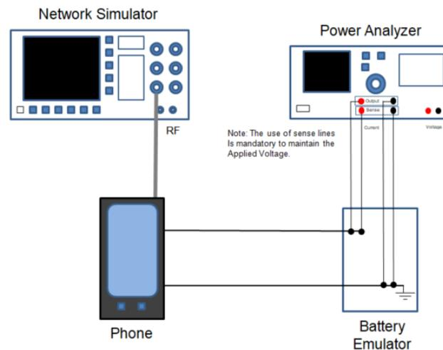
Figure 4.1-1 Energy Use Per Activity Test Setup
