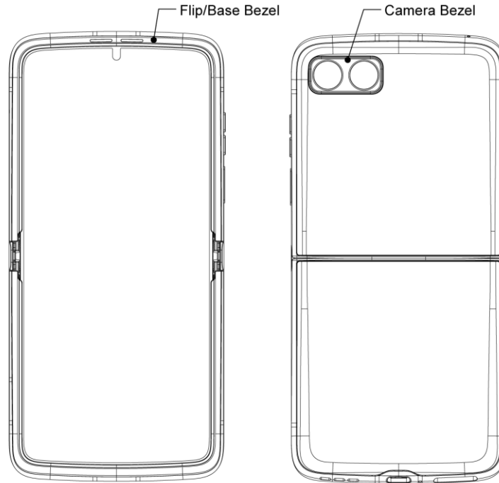
Figure 2.3-7 : "A" Surface Example for Foldable Devices
