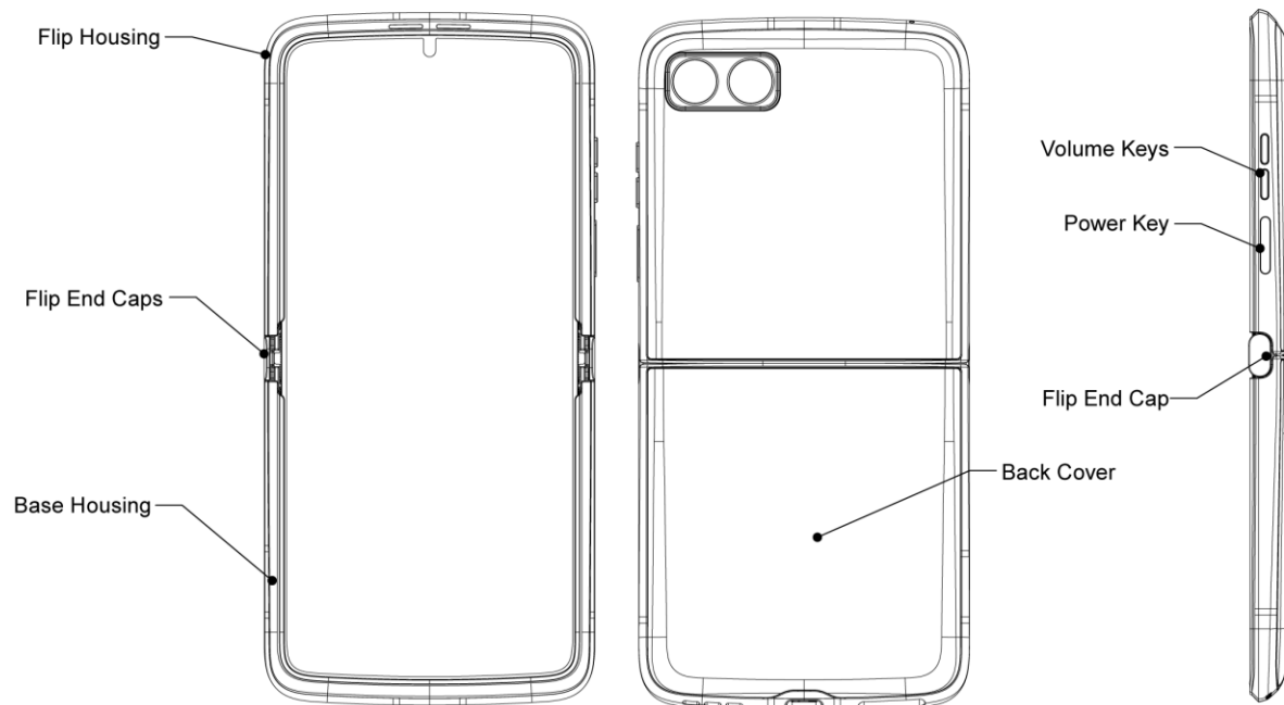
Figure 2.3-14 "B" Surface Example for Foldable Devices
