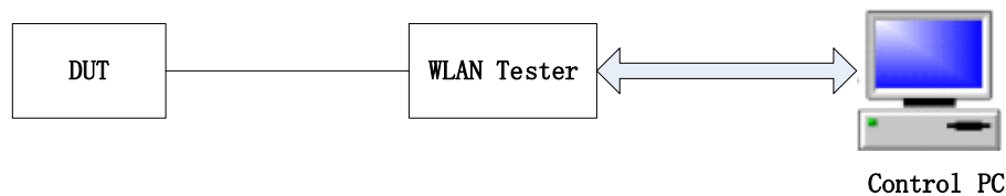
Figure 3.1.2-1 Block Diagram for Wi-Fi Conducted Measurement
